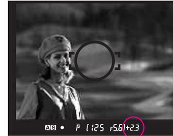
Keep pressing the AEL button **A**, and the difference between the metered exposure value and the exposure of the new composition will be displayed on the viewfinder LCD. This function can be used to see if an object of very different brightness levels can be properly photographed.
