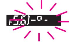
★ If the difference between the set value and the metered value exceeds 6EV, the viewfinder LCD blinks " - 0 - " for underexposure and " - 0 - " for overexposure.
