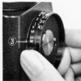
For instance, when using the 127mm f/3.8 or 90mm f/3.8. set 3.8 of the lens speed scale (4) opposite the index (3)
